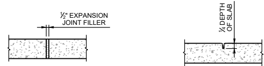
(A) EXPANSION JOINT (B) CONTRACTION JOINT
