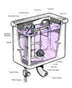
Water Closet with properly functioning Air Break
