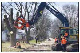
A rubber tracked excavator equipped with a special cutting shear moves the trunk of an ash on Orchid Lane.
