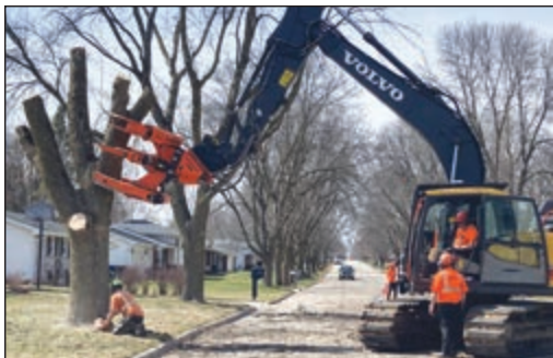
A rubber tracked excavator equipped with a special cutting shear moves the trunk of an ash on Orchid Lane.
